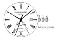
In addition to the regular functions of a mechanical watch, the moon phase rotates clockwise, completing a full cycle in 29.5 days.
